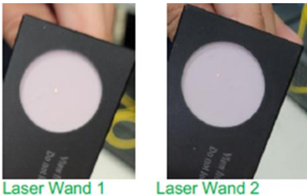
Figure 7. Two IR detection wand prototypes show visible fluorescence when exposed to 0dBm IR excitation source.
