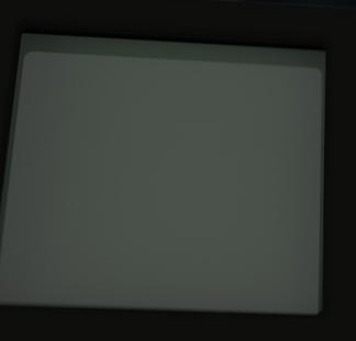
Illuminate from THIS side Detects wavelengths 1460-1600nm
