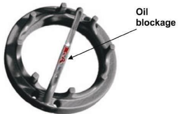
Figure 12—(d) A cutted into neutron tomogram of a of a helicopter engine lubricator revealing the blockage
