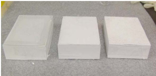
Fig. 1 Air brushing, liquid brushing, dry spreading ZnS(Ag) sensors, left to right
