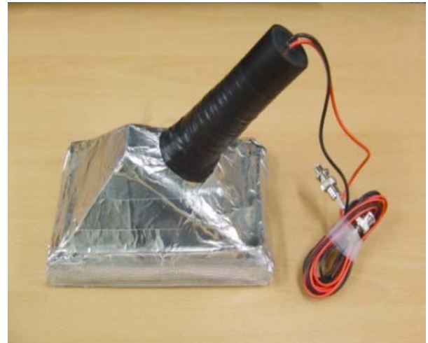
Fig. 7 New-method ZnS(Ag) alpha-particle detector probe.
