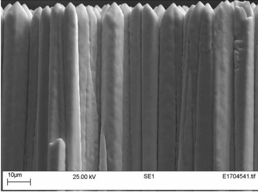
Scintacor's micro-columnar CsI as seen in a Scanning Electron Microscope
