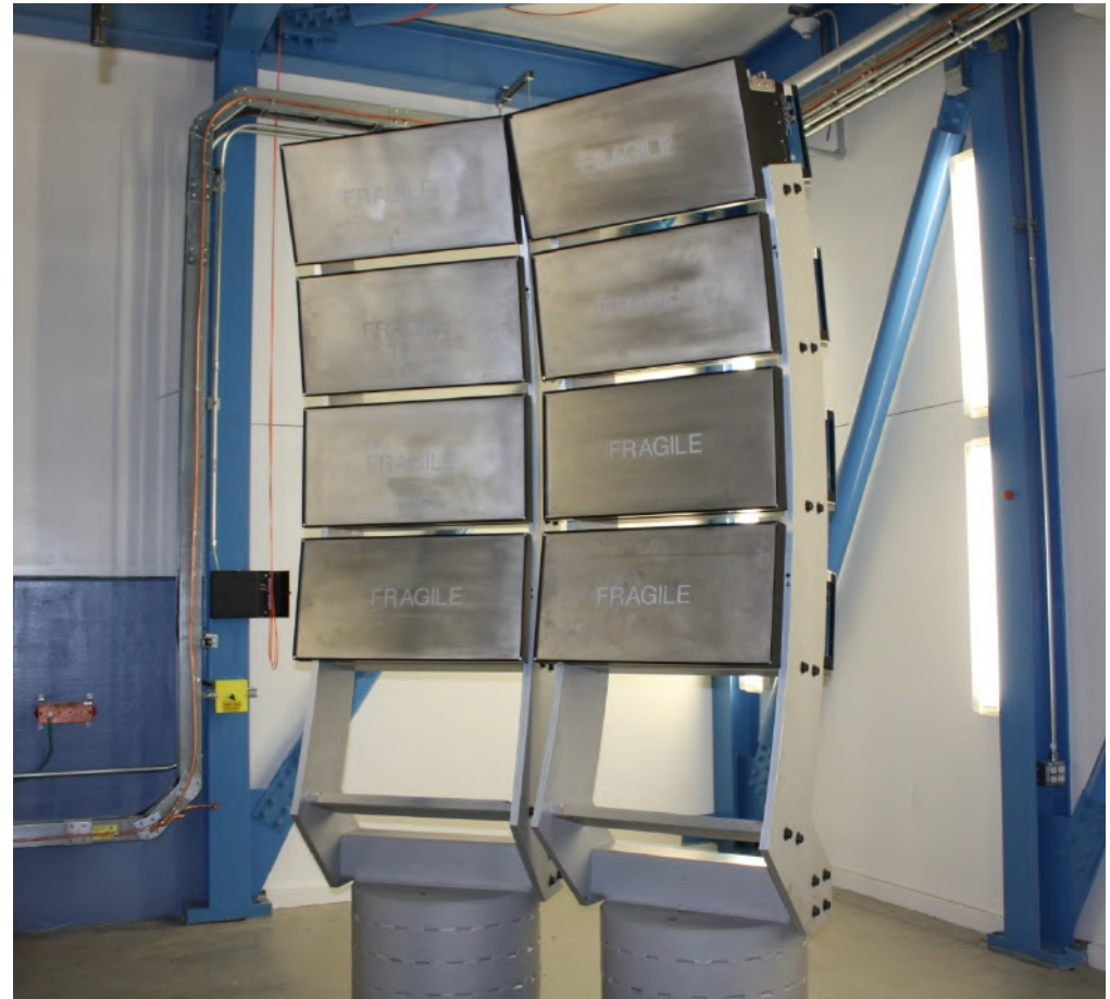
8 Detector array in POWGEN Instrument at SNS
